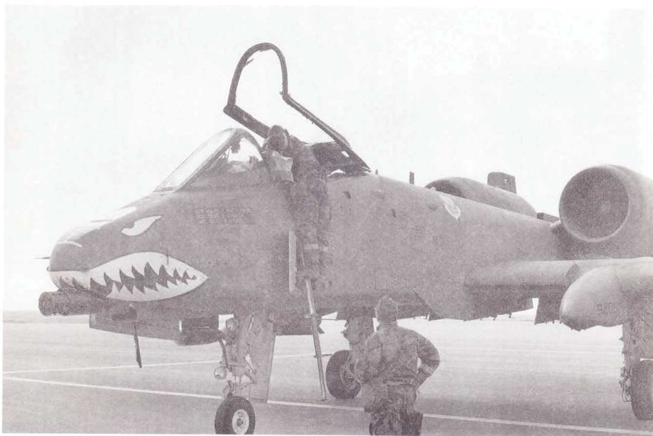
Figure 3 - 23d Tactical Fighter Wing A-10--its GAU-8/A 30mm anti-tank gun is clearly visible mounted in the nose section of the fuselage.
